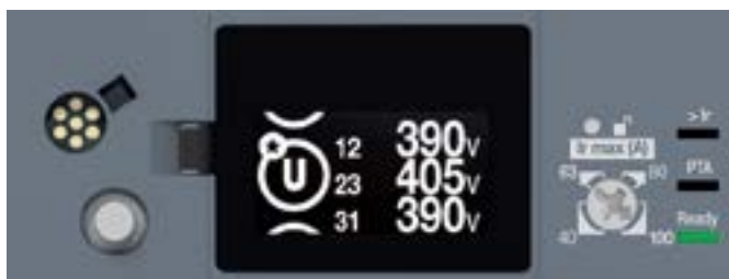
Embedded display Measurements menu
